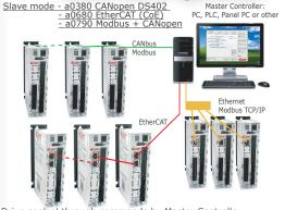
Drive control through commands by Master Controller. Suitable for multi axes systems.
